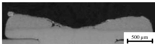
Figure 12: Micro section of Ag/SnO 2 12TOS (movable contact: anode) under load IIb (90 A / 30 A / 0.125 mH) first failure after 5.6 (relative factor)
