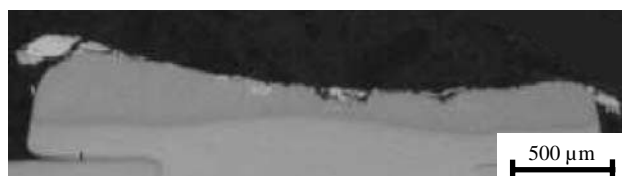
Figure 13: Micro section of Ag/SnO 2 12TOSF (movable contact: anode) under load IIb (90 A / 30 A / 0.125 mH) first failure after 10.5 (relative factor)
